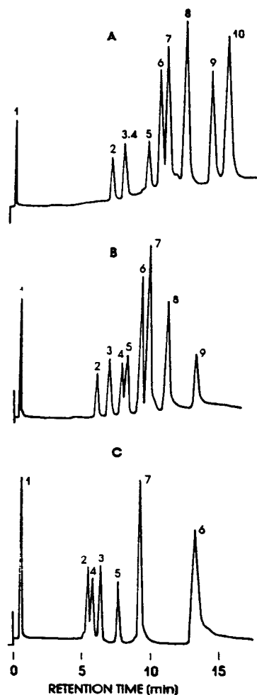
Fig. 4. Effect of mobile phase pH on separation of proteins. Column: 35- \mu m fluorocarbon resin, 8 cm \times 6.2 mm I.D. Mobile phase: Buffer to acetonitrile-buffer solution (70:30, v/v) in 20 min at 2 ml/min. Detection: UV at 220 nm. (A) 0.1% Trifluoroacetic acid, pH 2; (B) 0.1 M sulfuric acid, pH 1. (c) 0.1% ammonium hydroxide, pH 11. Peaks: 2 = enkephalin (leucine); 3 = enkephalin (methionine); 4 = insulin chain A; 5 = angiotensin I; 6 = ribonuclease; 7 = insulin; 8 = lysozyme; 9 = carbonic anhydrase; 10 = ovalbumin. From ref. 26.
